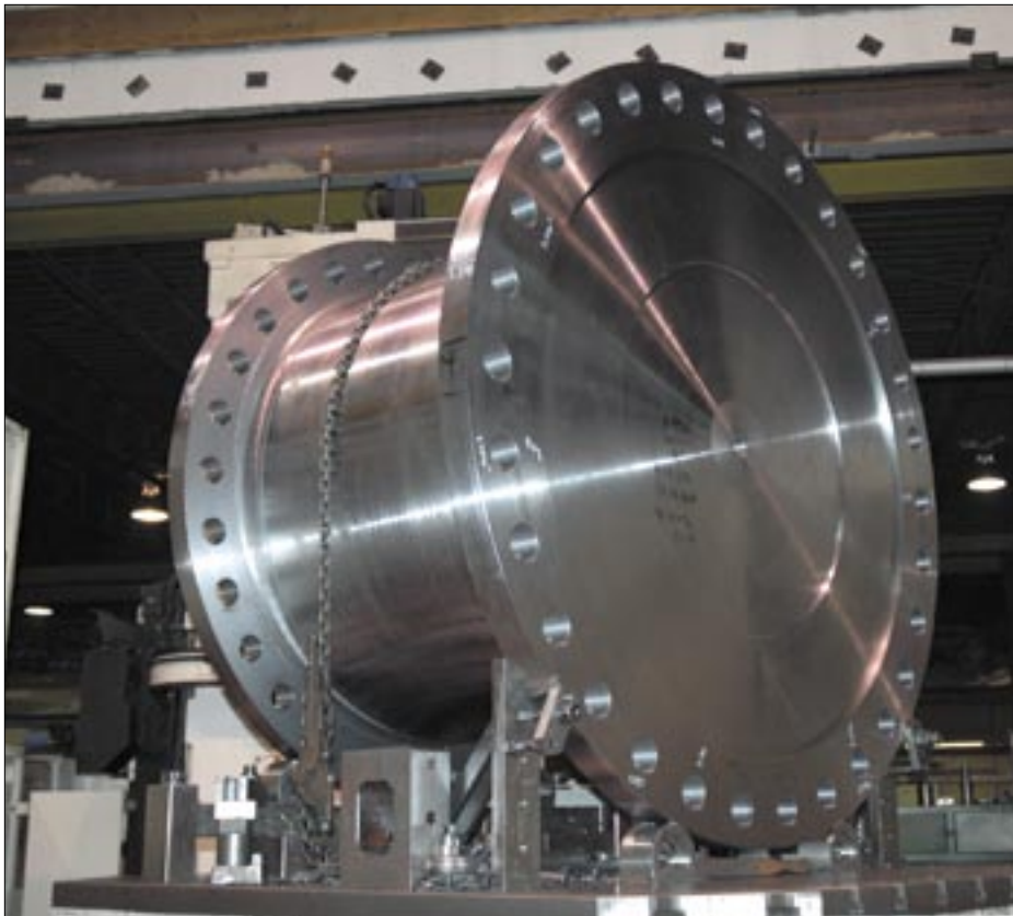
Finished machined large Steel Mill coupling drive spacer.
